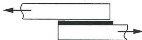
e. Adhesive Failure (Shear)
