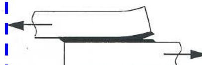
d. Cohesive Failure (Peel)
