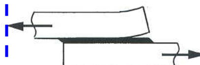
f. Adhesive Failure (Peel)
